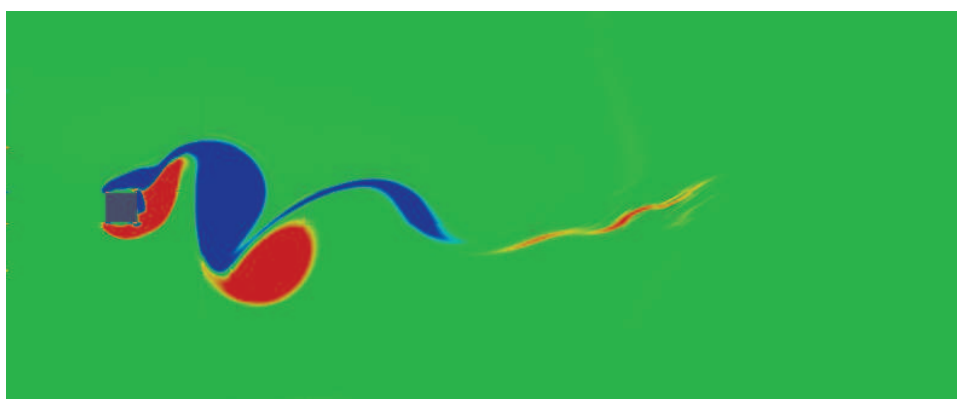
Figure 4.36: Vorticity flow past a rectangle. Solution at instant T = 20.5s computed with the 2 level SWR implicit scheme. The unit square is closer to the border, at position [2, -.5] .
