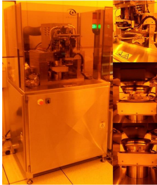
Figure 5.17. Obducat Nano Imprint Lithography EITRE machine
