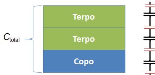
Figure 3.20. Electrical schematic representation of multilayer (sample multi-P-3) with material capacitors connected in series including interface capacitance (in red).
