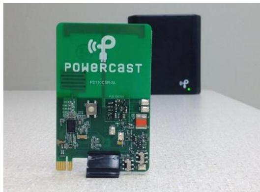
FIGURE 1.5 – P2110CSR Powerharvester® Wireless Sensor Card de Powercast [www.powercastco.com]
