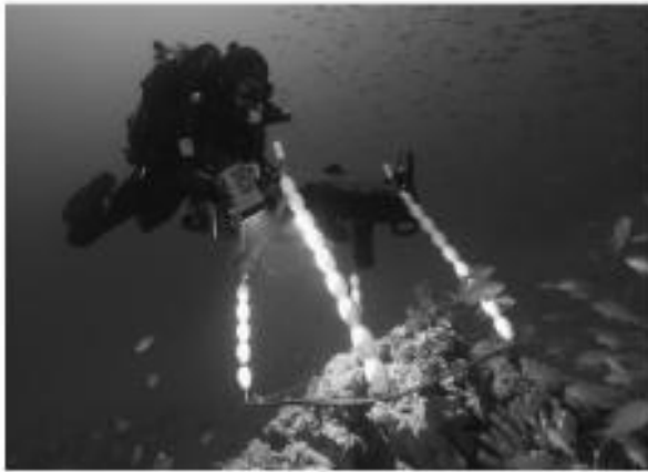
Fig. 3. Photographic quadrat system used in the field. A digital camera was perpendicularly fixed 30 cm over the quadrat frame.
