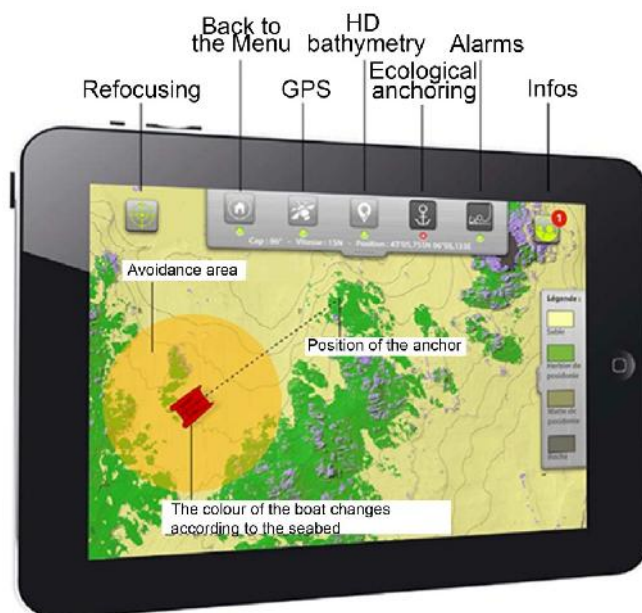
Figure 1: Main window of DONIA® application (currently only available in French). The legend displays color correspondence for the habitats: yellow = sand, green = Posidonia oceanica meadow, brown = dead matte and violet = rocky habitat.
