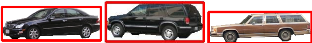
Figure 6.6: Exemples de rectangles minimums englobant
