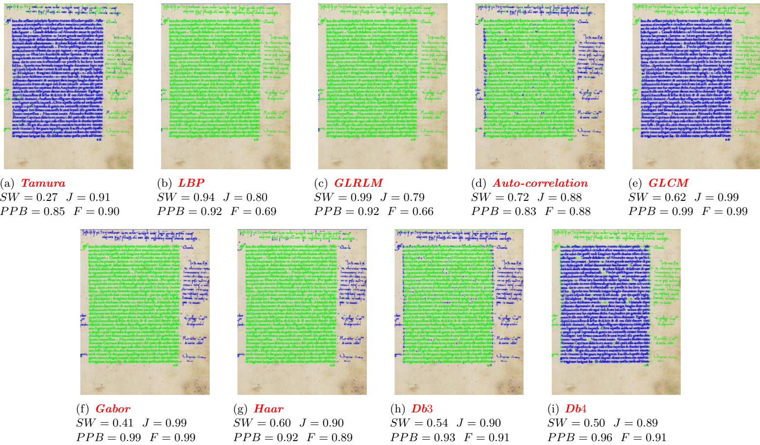
Figure 4.11.: Examples of resulting images of the proposed pixel-labeling scheme for comparing the nine investigated texture-based feature sets on the “Only two fonts” category of HDIs from the “DIGIDOC-Texture dataset” . Since the process is unsupervised, the colors attributed to text or graphics may differ from one DI to another.
