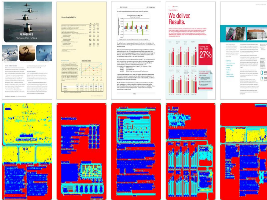
Figure 3.21.: Result examples of a texture-based approach for pixel classification of business DIs proposed by Cote and Albu [3].
