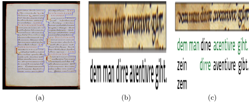
Figure 2.23.: Illustration of the three complementary modules of the HisDoc project. Figures (a), (b) and (c) show the HDI layout analysis, handwritten text recognition and information retrieval modules, respectively 70 [34].
