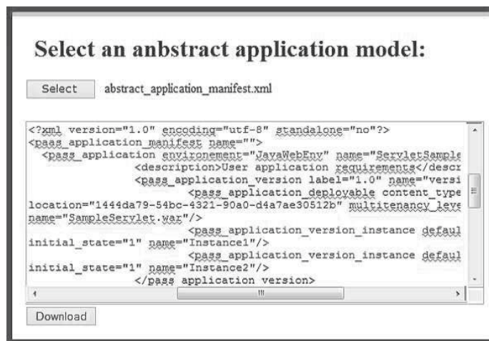
Figure 6.4: Screenshot of the interface allowing to import the abstract application manifest and generate the deployment manifest
