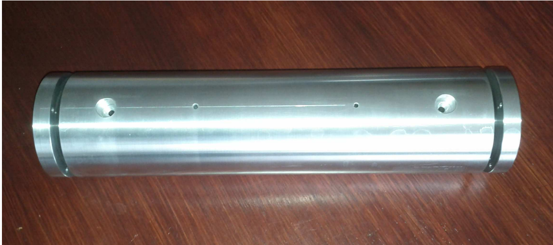
Figure 6.1 Most recent ring-down cavity machined in a monolithic aluminium cylinder. Mirrors, O-rings, adjustment screws and PZT-assembly are not yet mounted on this photography.
