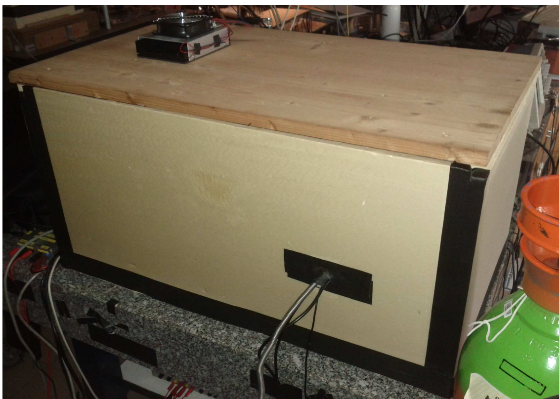
Figure 6.5 Peltier-stabilized polystyrene enclosure containing the OFFS-CRDS setup.
