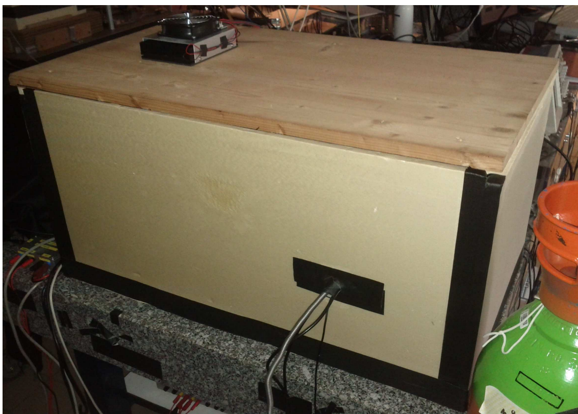
Figure 6.5 Peltier-stabilized polystyrene enclosure containing the OFFS-CRDS setup.
