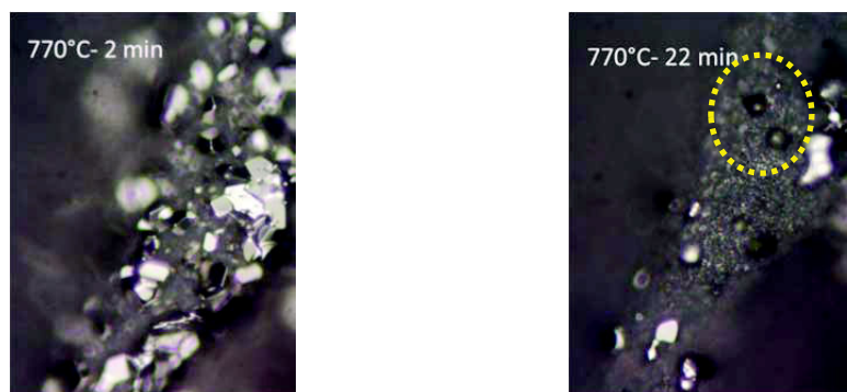
Figure 24. In situ images of nickel sulfide crystals at 770°C in 500 ppm H 2 S as a function of time. Yellow circles indicate the appearance of black round shapes
