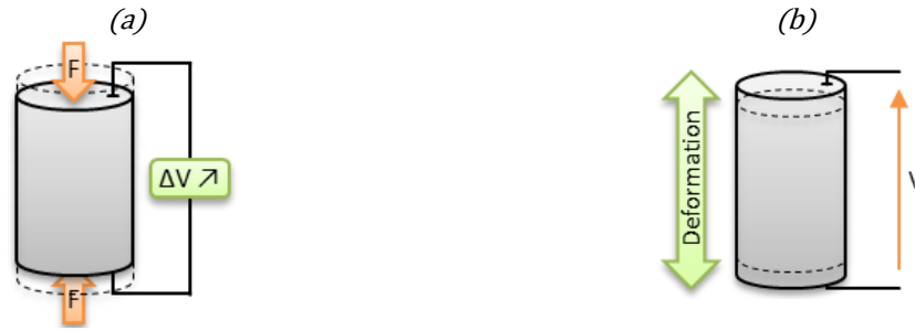
Figure 2 Schematic of the (a) direct piezoelectric effect and (b) inverse piezoelectric effect.
