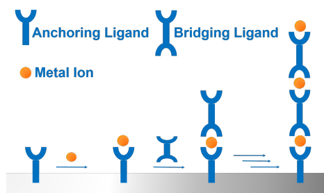
Figure 2.1: A schematic representation of the stepwise (layer by layer) preparation of surfaces
