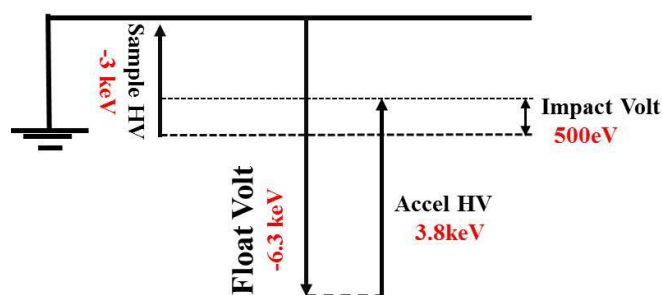
Figure II-16 Illustration of the principle of work of floating column.
