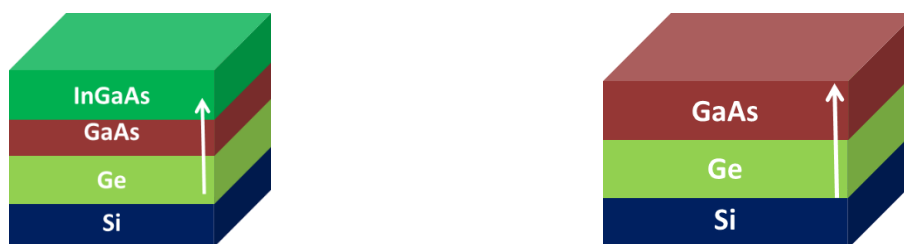
Figure II-8 Structure of InGaAs/GaAs/Ge/Si (IGA #1, 2, 3) and GaAs/Ge/Si (GaAs ref #12) samples grown on Si substrate.
