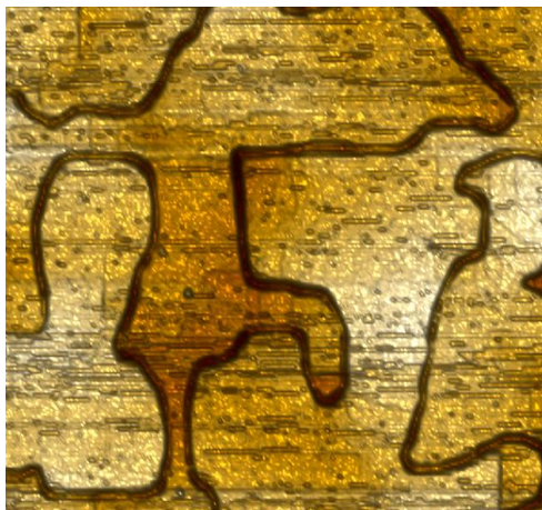
Figure IV-20 Initial topography of III-V heterostructures grown on planar Si wafers, -, nm, scanning zone 3.3 \mu m \times 3.3 \mu m , where 14.8 \text{ nm} < z < 7.8 \text{ nm} .
