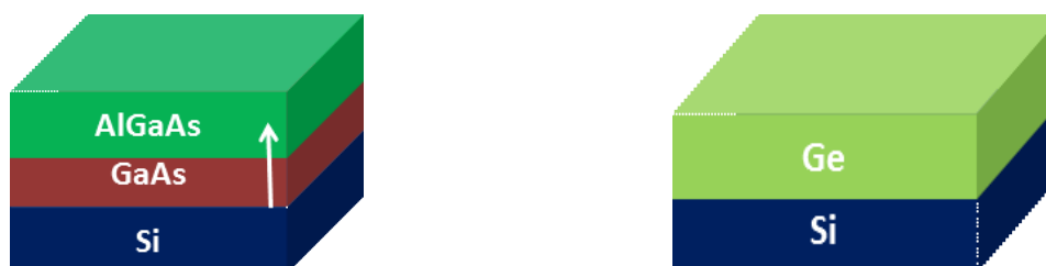
Figure II-9 Structure of AlGaAs/GaAs/ Si (AlGa #13) and GaAs/ Si (GaAs ref #14) samples grown on Si substrate.
