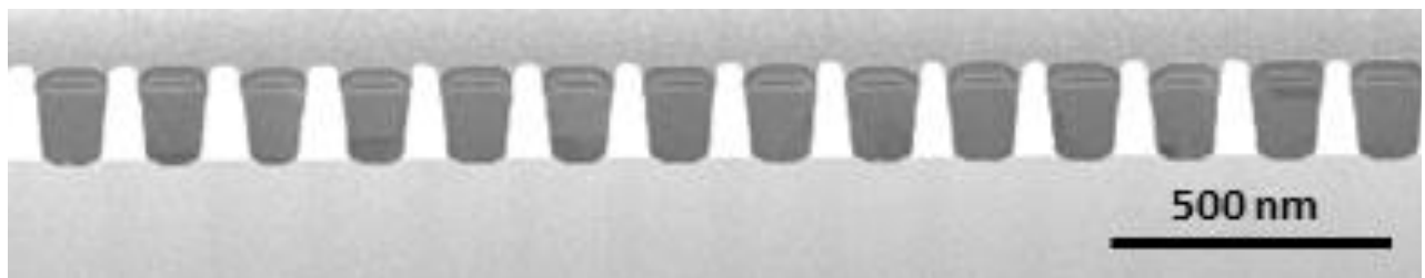
Figure IV-1 A cross-section STEM image of III-V heterostructures selectively grown in cavities on 300 mm Si wafers using the aspect ratio trapping method.
