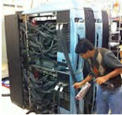
FIGURE 2.2 – Emulateur Palladium supportant 256M de portes
