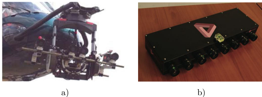
Fig. 5.25: a) 4 camera rig used by Binocle in the shooting of “La France entre ciel et mer” (France between sky and sea). b) 8 camera rig proposed by PrevotEAU et al. (2010) .
