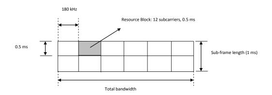
Figure 5.2 – LTE Frame Structure in Frequency Domain
