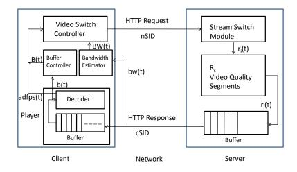
Figure 4.1 – Adaptive Streaming Architecture
