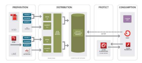
Figure A.2 – Preparation, Distribution, Protetionc and Consumption of HDS [39]
