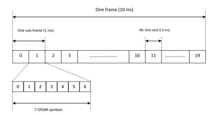
Figure 5.3 – LTE Frame Structure in Time Domain
