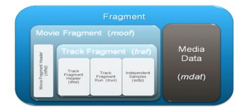
by the client player. The requested fragment of the file is sent to the client over the wire, hence the name 'wire format'. The format of fragment is shown in Figure A.4.
