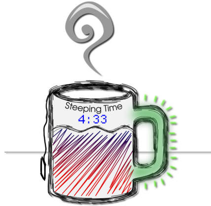
Figure 2: A sketch of an augmented mug. It displays the remaining steeping time for a perfect cup of tea. The overlay shows the quantity and temperature of the liquid inside. The handle will glow green when the tea is ready and that the temperature is appropriate to avoid nasty tongue burns.
