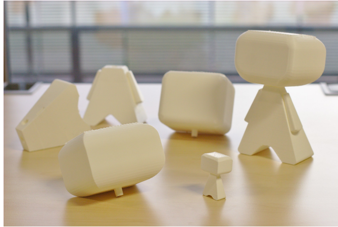
Figure 54: Modular 3D printed body pieces in order to quickly create a personalized Tobe.
