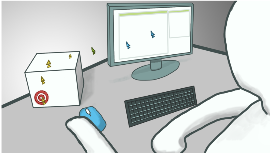
Figure 22: A sketch describing a standard desktop environment which would allow a mouse pointer to travel out of the screen and into the surrounding environment to acquire targets.
