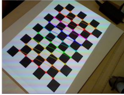
Figure 18: A chessboard typically used in camera calibration. The physical size of the squares are known and can be automatically detected using computer vision.
