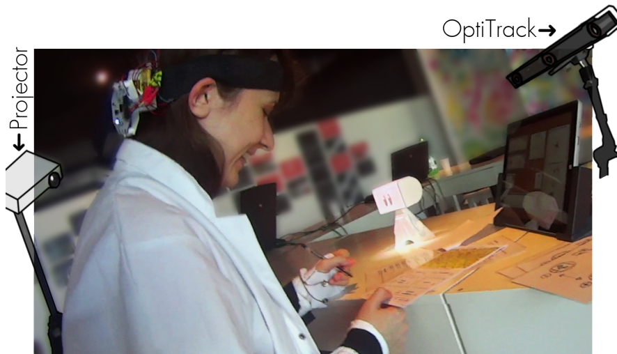
Figure 55: In a scientific museum, various activities were proposed to visitors in order to prompt self-investigation. The setup consists of a projector handling the augmentation and an OptiTrack for the tracking.
