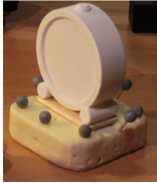
Figure 17: Multiple reflective balls are attached to an object's base. IR light is shed on them and tracked by multiple IR cameras.
