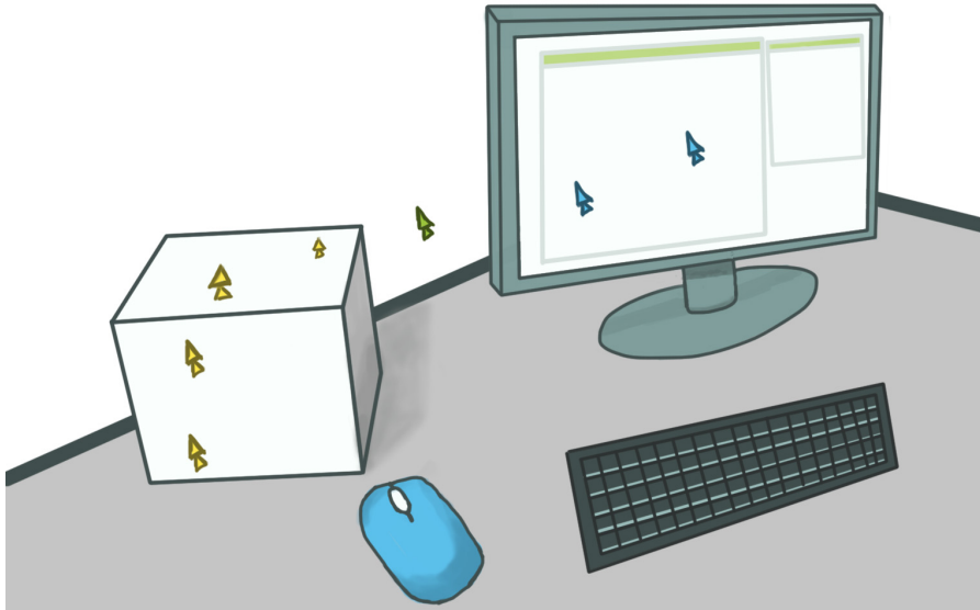
Figure 32: An augmented object is located beside a screen. When the cursor reaches the edge of the screen, it “leaks” out in the environment.
