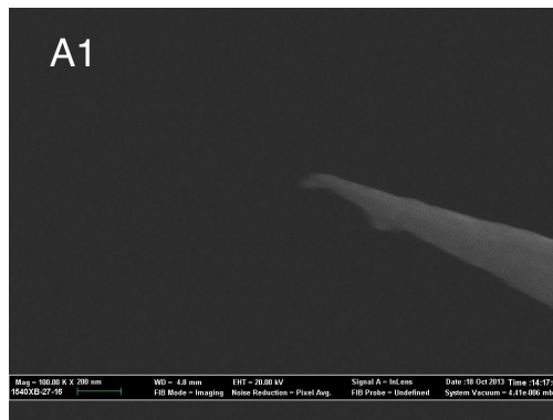
Figure B.3 – SEM image of tip A1 before laser irradiation. No SEM image of tip A1 after laser irradiation. The sample kept charging up making imaging impossible.
