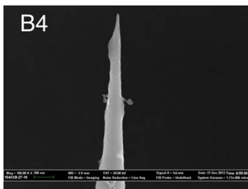
Figure B.12 – SEM image of tip B4 after laser irradiation. No SEM image of tip B4 before laser irradiation. Sample kept charging up making imaging impossible.
