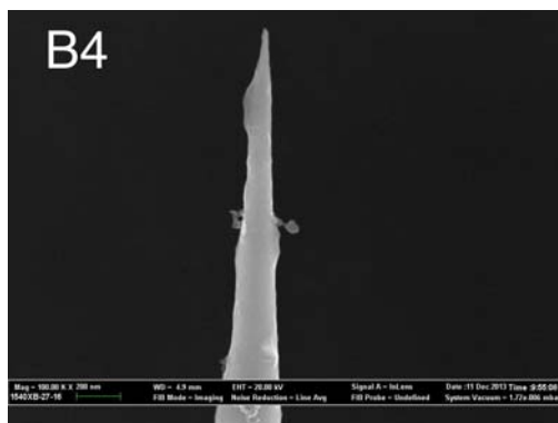
Figure B.12 – SEM image of tip B4 after laser irradiation. No SEM image of tip B4 before laser irradiation. Sample kept charging up making imaging impossible.
