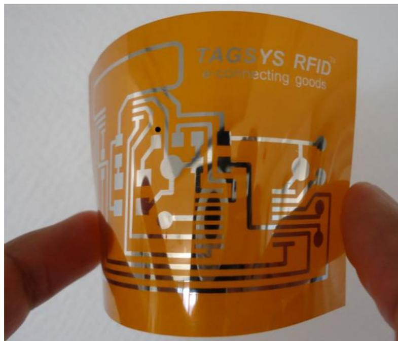
**Figure 1.1:** Inkjet-printed circuit on flexible polyimide substrate.
