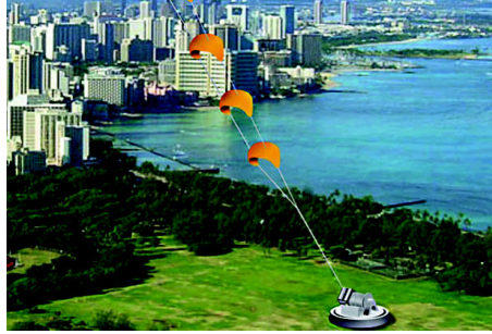
Figure I.12: Imagined laddermill of Delft University of Technology
