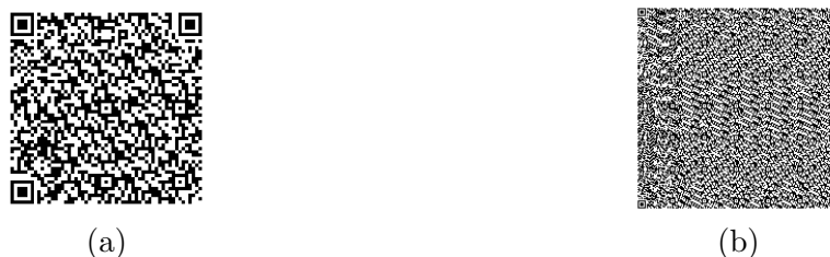
FIGURE 6.1: QR code evolution: a) QR code V10 with 57 \times 57 modules, b) QR code V40 with 177 \times 177 modules.
