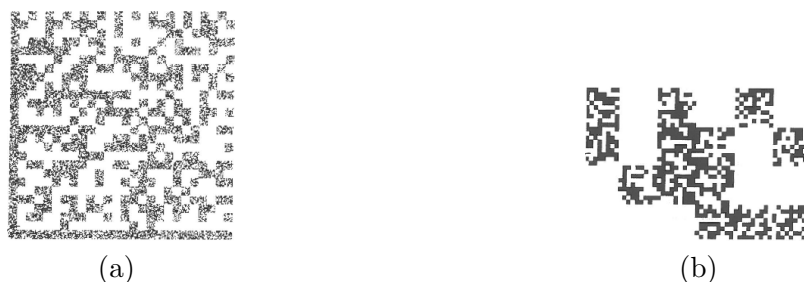
FIGURE 4.22: Examples of barcodes with authentication property [109]: a) DataMatrix with replaced black modules by CDPs, b) Zoom of DataMatrix (a).
