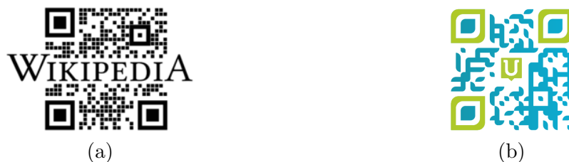
FIGURE 4.4: Examples of design QR codes: a) Replacement of modules by logo 2 , b) Change of module shape, colors and logo insertion 3 .
