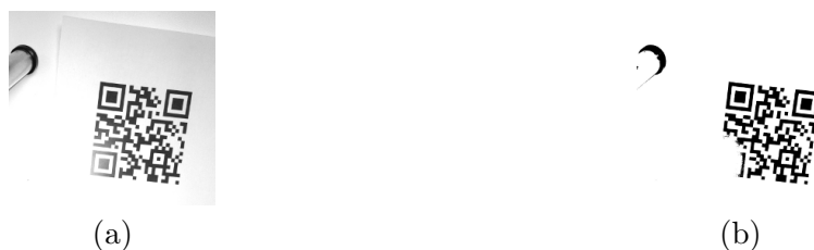
FIGURE 6.3: An example of: a) QR code under non-uniform lighting conditions, b) binarization results using standard global thresholding method.
