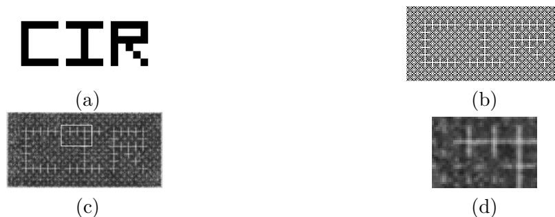
FIGURE 5.16: Example of textured images containing a visual message: a) Binary visual message, b) Textured image containing the visual message (a), c) P&S textured image (b), d) Zoom of central part of P&S textured image (c).
