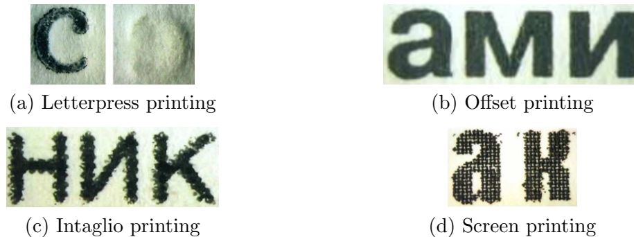
FIGURE 2.2: Examples of characters printed using 1 : a) Letterpress technique, b) Offset technique, c) Intaglio technique and d) Screen printing.
