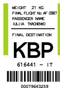
FIGURE 4.1: Example of 1D barcode into baggage ticketing.
