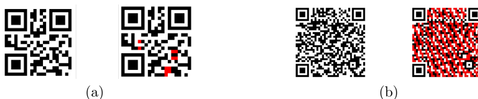
FIGURE 4.15: Examples of QR codes with hidden information (in both images red modules correspond to changes added to QR code): a) QR code V1, low error correction level, before and after message hidden by method [83], b) QR code V5, high error correction level, before and after message hidden by method [20].
