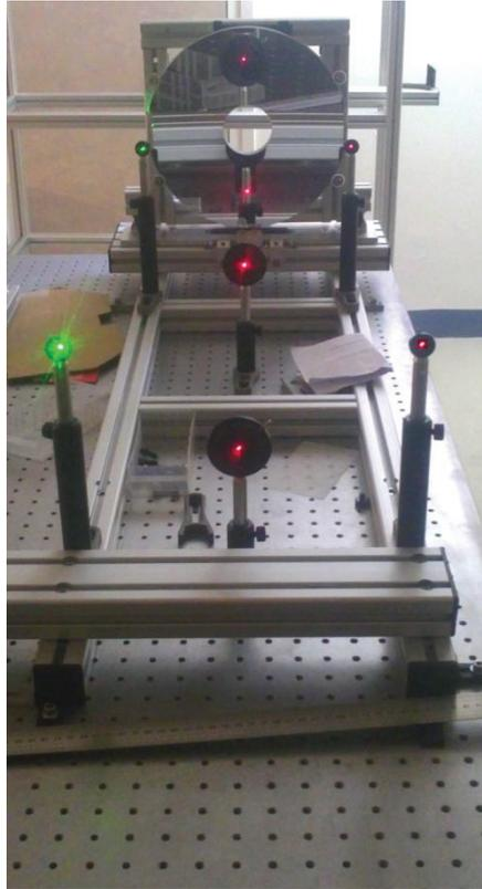
**Fig. 5.21:** The 30 cm diameter telescope during the alignment procedure.
