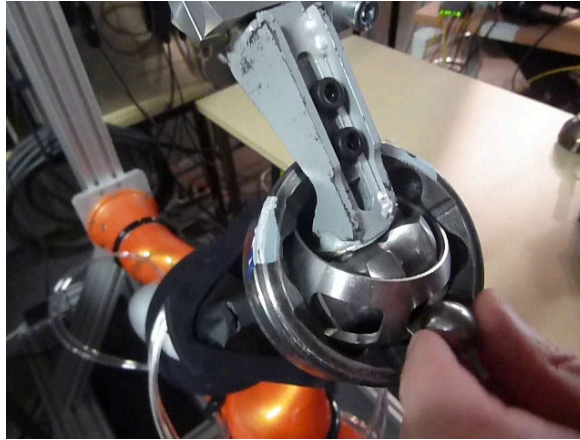
Figure 5.16: The hand of the human gets close to the outer shell when inserting a ball. If the robot moves unexpectedly at this moment, the human fingers may be injured.
