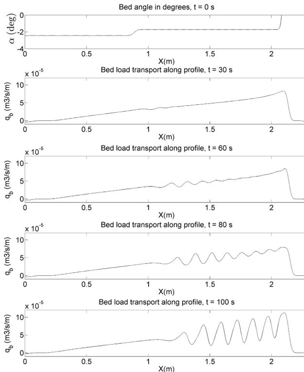
FIGURE 4.10 – Initial bed slope angle ( $\alpha$ ) and bed load transport ( $q_b$ ) along the dune profile from  $t = 30$  s to  $t = 100$  s for an idealized dune presenting a  $1^\circ$  deflection in its stoss side slope.
