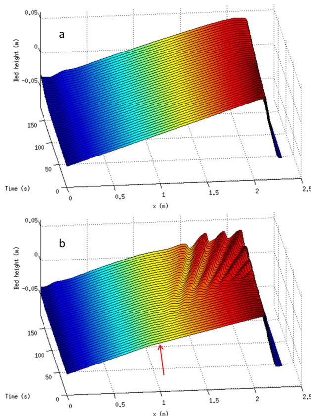
FIGURE 4.9 – (a) Time evolution of an idealized triangular-shaped dune and (b) time evolution of an idealized triangular-shaped dune presenting a deflection of  $1^\circ$  (pointed by a red arrow) in the stoss side slope. The vertical scale is exaggerated 10 times and the red arrow shows the position of the slope deflection.
