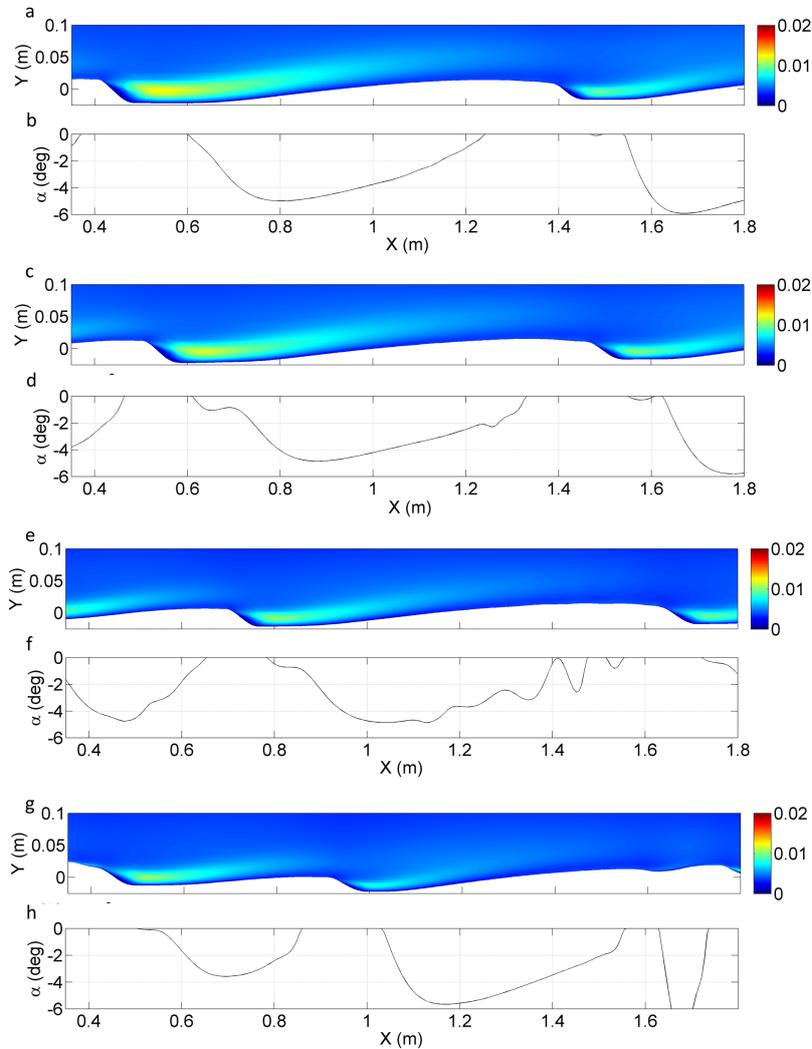
FIGURE 4.12 – Deflection shifting sequence with (a), (c), (e), (g) the turbulent kinetic energy field,  $k$ , and (b), (d), (f), (h) the bed slope along the bed profile,  $\alpha$ , at  $t = 1850$  s,  $t = 2000$  s,  $t = 2300$  s, and  $t = 2650$  s respectively. Higher values at the crest are not shown for a better visualization.
