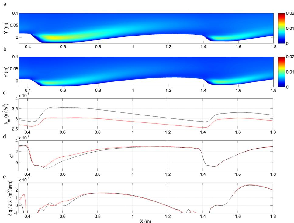
FIGURE 4.11 – (a) Turbulent kinetic energy field  $k$  at  $t = 1850$  s for the baseline simulation (scenario 1) and (b) with a 25% lower upstream dune (scenario 2) with the corresponding spatial evolution of (c) the mean turbulence in the water column  $k_m$ , (d) the skin friction coefficient  $c_f$ , and (e) the total transport gradient  $\Delta q / \Delta x$  for scenario 1 (black) and scenario 2 (blue).
