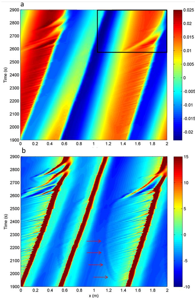
FIGURE 4.8 – Time evolution of (a) the bed height, and (b) the bed slope (in degrees) from the zoomed-in subset in Figure 4.4. The red arrows indicate the position of the dune stoss slope deflection.
