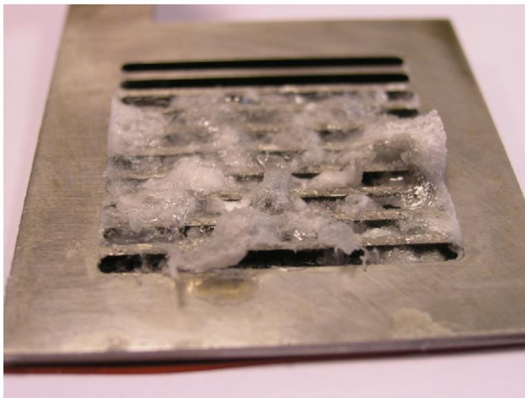
Figure 8: Photograph of the air cathode current collector after long-term operation of a DBFC. Reproduced from Ref.[46] with permission from Elsevier.
