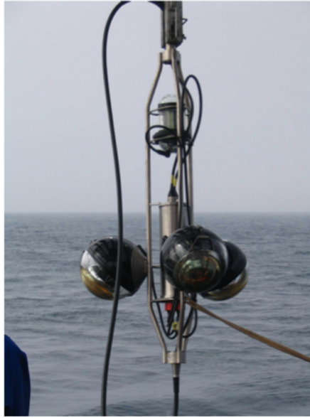
Figure 2.7: Picture of a storey being deployed. There are 3 /acOMs facing 45^\circ downward, and the LCM in the center housing the readout electronic cards. A LED optical beacon for timing calibration purposes can also be seen in the top part of the storey frame.
