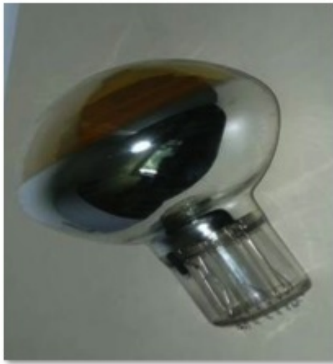
(a) Design 1 : 40° photocathode maximum zenith angle for prototypes 1 and 2
