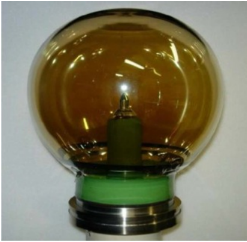
(a) CERN X-HPD prototype
