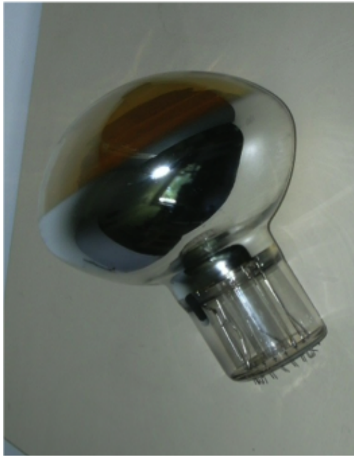
(a) CPPM-Photonis prototype without the rear small photomultiplier.
