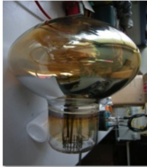
(b) Design 2 : 60° photocathode maximum zenith angle for prototype 3
