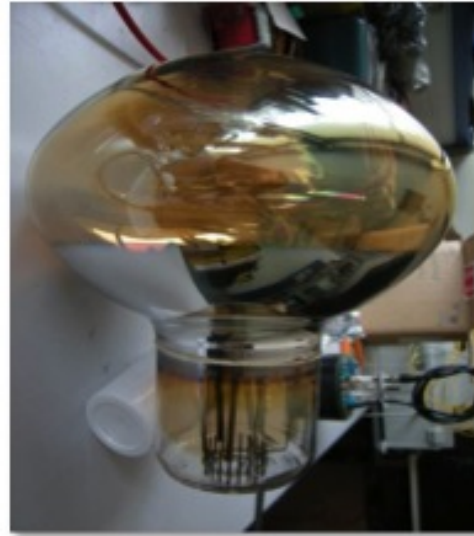
(b) Design 2 : 60^\circ photocathode maximum zenith angle for prototype 3
