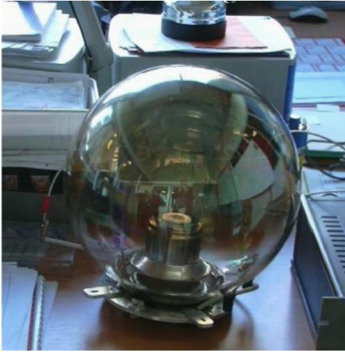
(a) The Philips XP2600 X-HPD, constructed at the Philips Brive la Gaillard site: now Photonis S.A.S.
