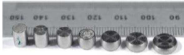
Fig. 1. Samples of HE material cold deformed at different rates.
