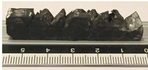
Figure 35: Broken sample by ECAP at low temperature.
