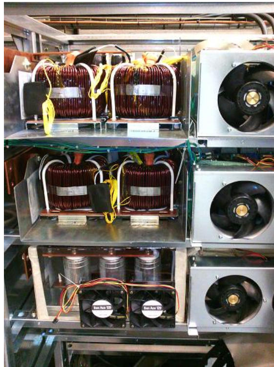
Figure 126: Interleaved legs filter solution
