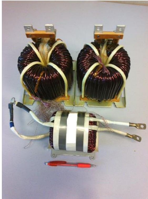
Figure 127: Interleaved chokes vs coupled solution
