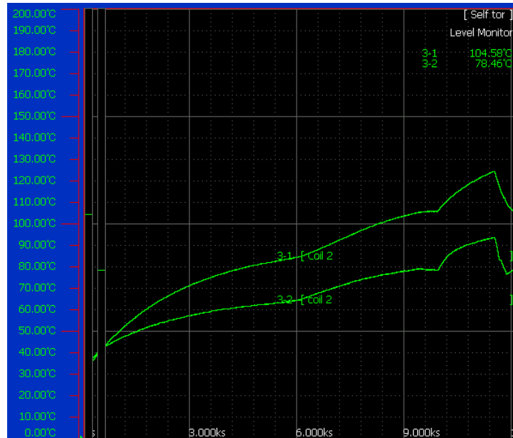
Figure 141: Temperature rise for nominal functioning with fault condition at the end, inner and outer coils temperature sensors
