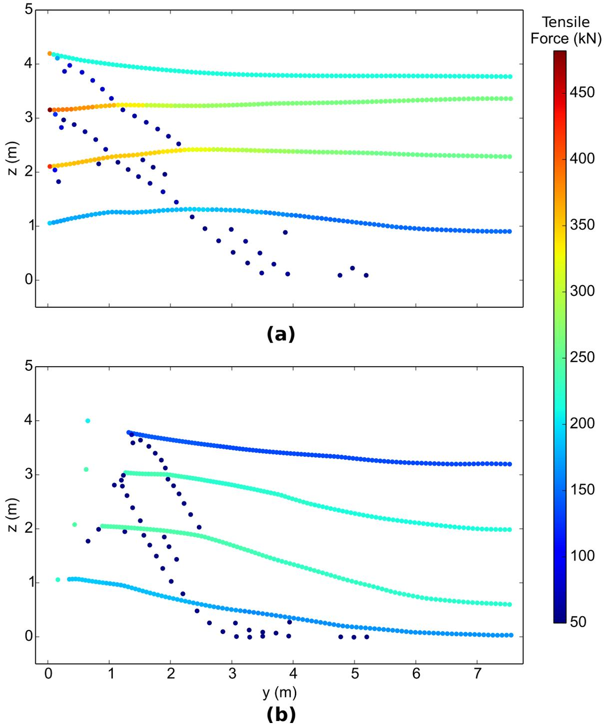
*Figure 4.25: Tensile forces larger than 50 kN in cylinders forming main cables and net elements: (a) flexible barrier without energy dissipators (fbNo), (b) flexible barrier with energy dissipators (fbEd)*
