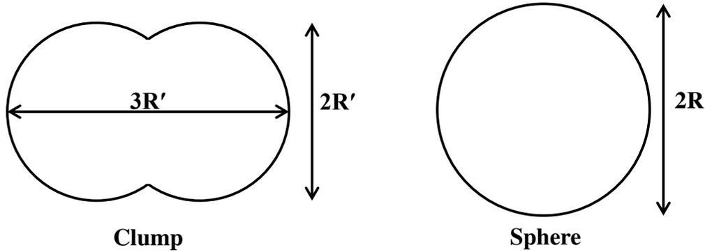
Figure 3.4: Particle shapes tested in the simulation: a clump and a simple sphere
