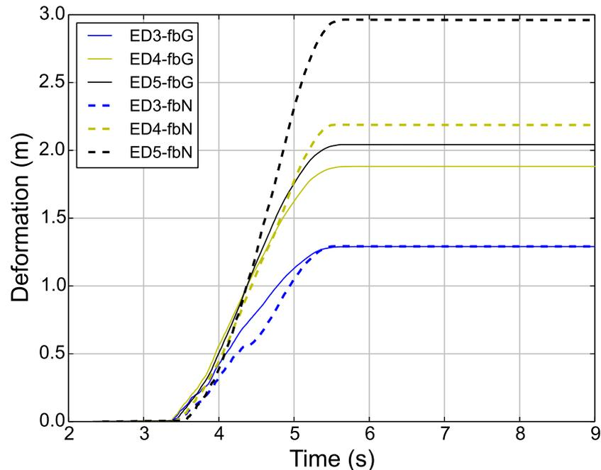
**Figure 5.16:** Evolution of deformation of energy dissipators installed on cables 3, 4 and 5 for two cases: a flexible barrier parallel to gravity vector (fbG) and a flexible barrier normal to channel base (fbN)
