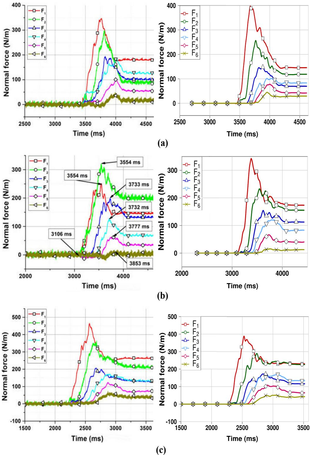
Figure 3.17: Time history of normal force variation: experiment (after Jiang and Towhata, 2013) (left) and model (right): (a) test L34-H15- $\alpha 45^\circ$  (b) test L44-H15- $\alpha 40^\circ$  (c) test L44-H20- $\alpha 40^\circ$
