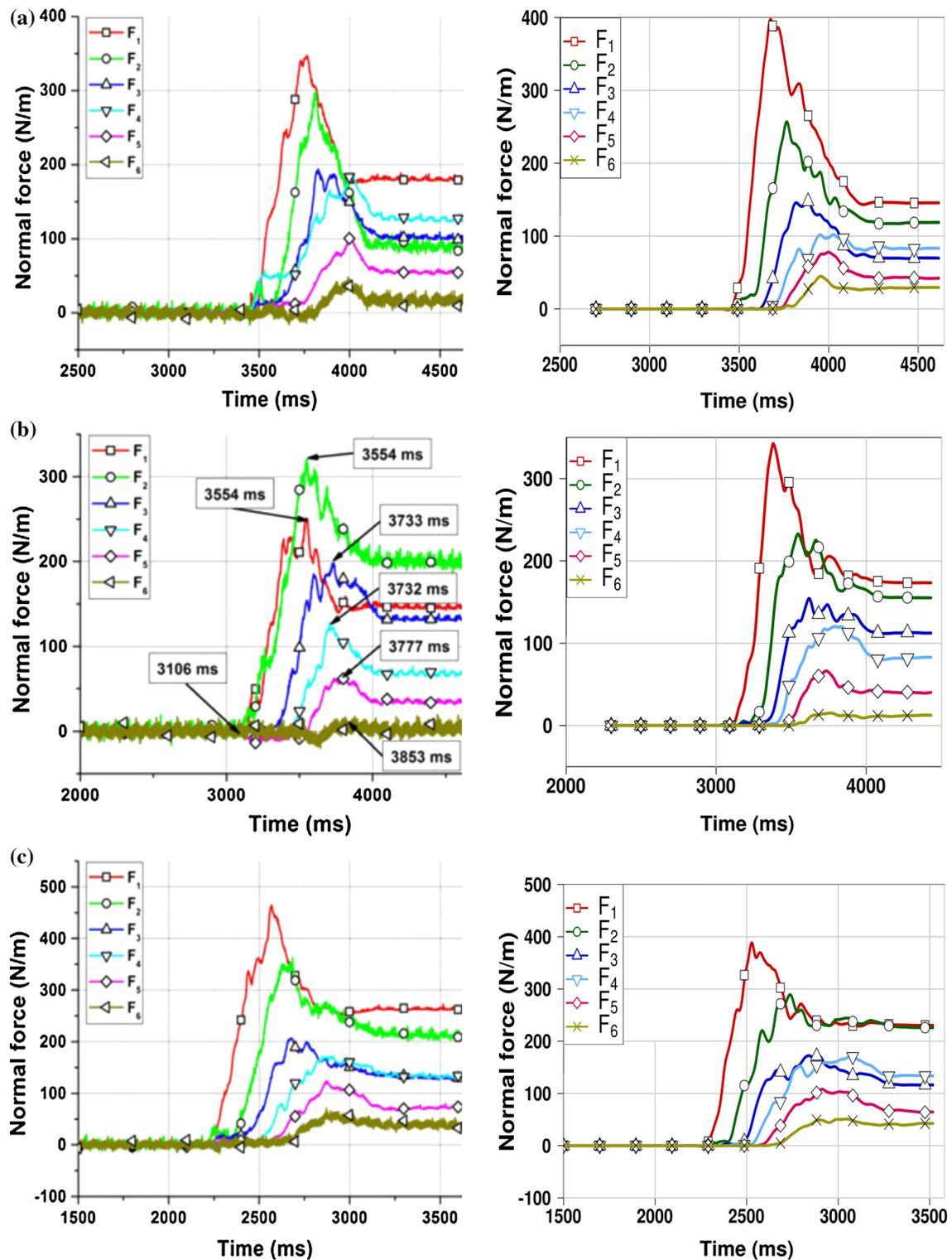
**Fig. 16** Time history of normal force variation: model (right) and experiment [23] (left): **a** test L34-H15- $\alpha 45^\circ$  **b** test L44-H15- $\alpha 40^\circ$  **c** test L44-H20- $\alpha 40^\circ$
