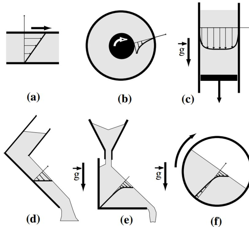
**Figure 2.1:** The six investigated configurations of granular flows: (a) plane shear, (b) annular shear, (c) vertical-chute flows, (d) inclined plane, (e) heap flow, (f) rotating drum (after [MiDi, 2004](#))
