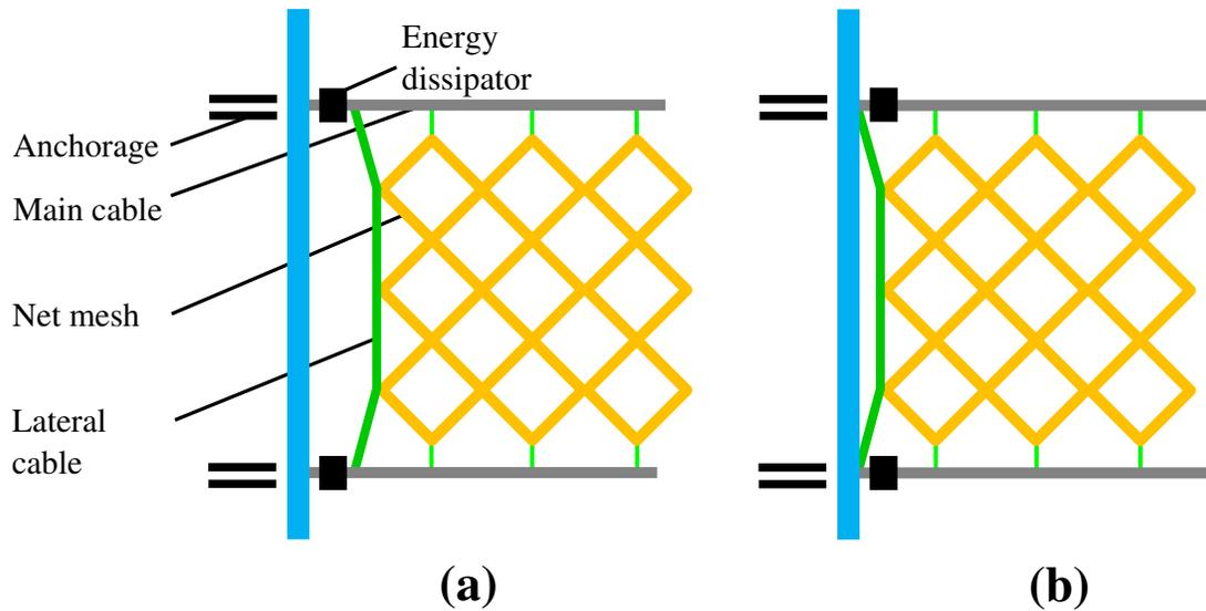
**Figure 5.17:** Schematic representation of two technologies for connecting the lateral cables: (a) lateral cables connected to energy dissipators ( $des_1$ ), (b) lateral cables connected directly to the anchors ( $des_2$ )
