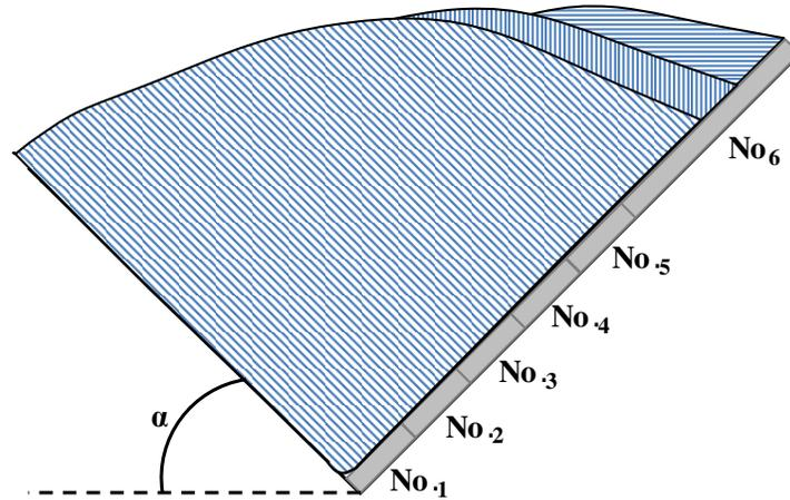
*Figure 3.6: Schematic representation of three different granular deposits (of same volume) showing the indirect relation between the final shape of the deposit and the residual force applied on the 6th segment of the wall*
