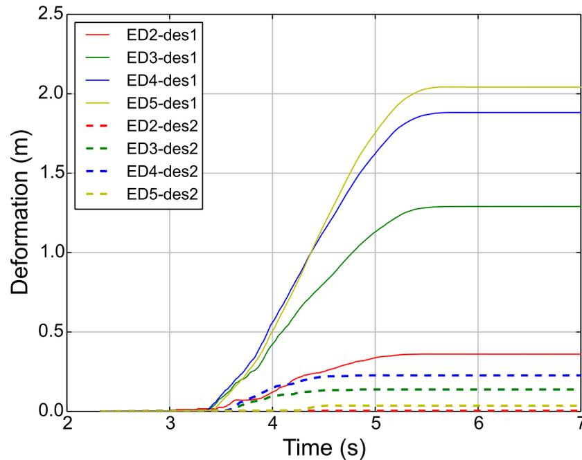
Figure 5.20: Evolution of the deformation of energy dissipators for two different configurations of the lateral cables: lateral cables connected to energy dissipators ( $des_1$ ) and lateral cables connected directly to the anchors ( $des_2$ )
