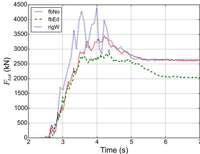
*Figure 5.7: Evolution of the total force applied by the flow, for three structures: a flexible barrier without energy dissipators (fbNo) and a flexible barrier with energy dissipators (fbEd) and a rigid wall (rigW)*
