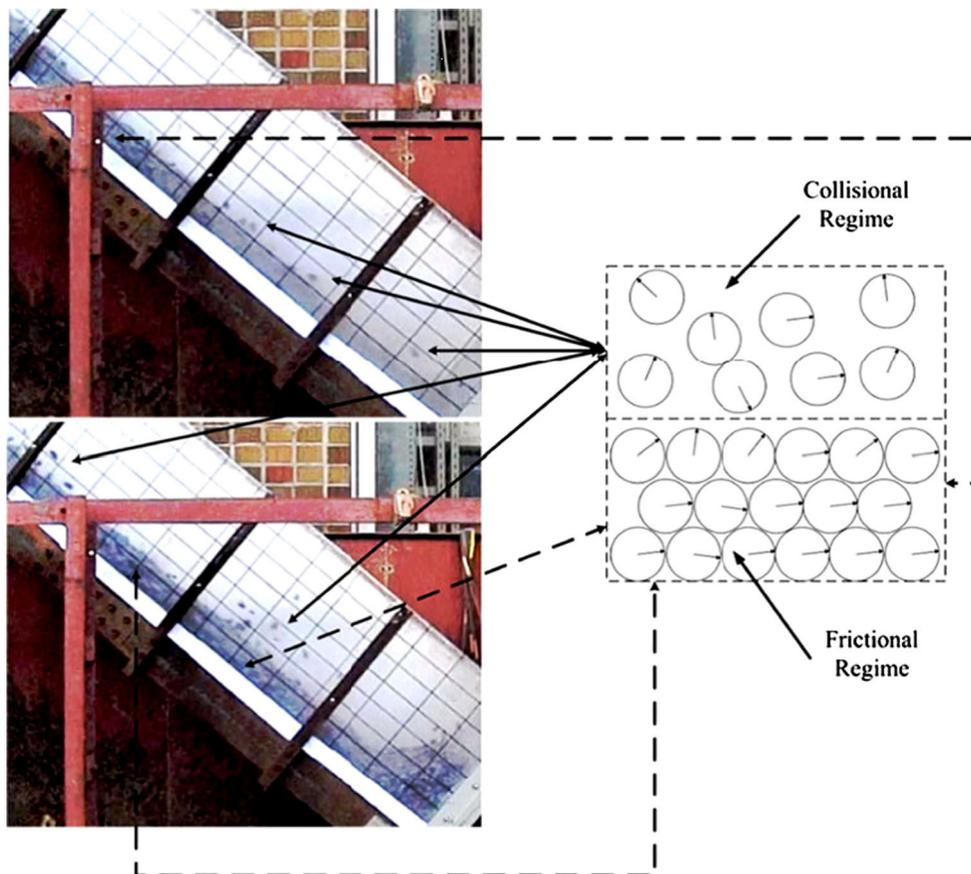
**Fig. 9** Snapshots of the experiment showing frictional and collisional regimes of the flow, *top*: before the impact, *bottom*: after the impact [23] (with permission of Springer Science+Business Media)
