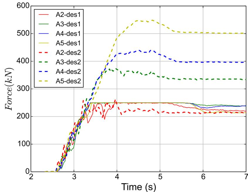
**Figure 5.21:** Evolution of forces applied on the anchors for two different configurations of the lateral cables: lateral cables connected to energy dissipators ( $des_1$ ) and lateral cables connected directly to the anchors ( $des_2$ )
