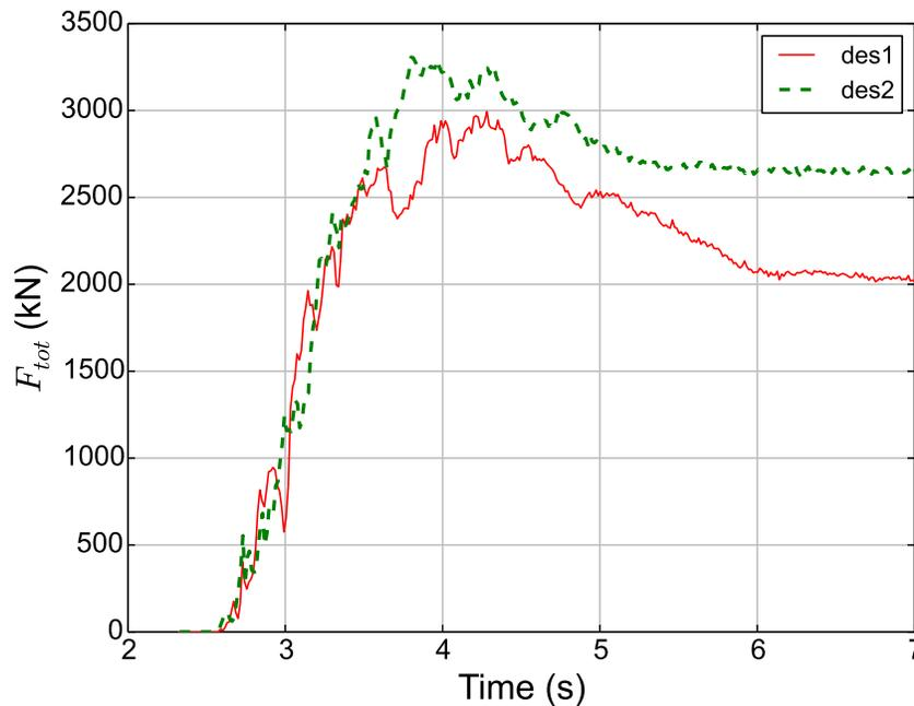
**Figure 5.18:** Evolution of total force applied on barriers with two different configurations of the lateral cables: lateral cables connected to energy dissipators ( $des_1$ ) and lateral cables connected directly to the anchors ( $des_2$ )
