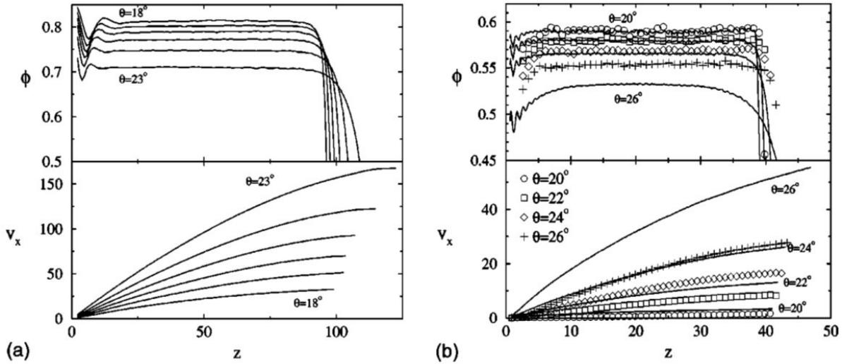
*Figure 2.2: Profiles of the solid fraction and the velocity in the direction of the flow, as a function of the distance from the channel base: (a) 2D simulation, (b) 3D simulation (after Silbert et al., 2001)*
