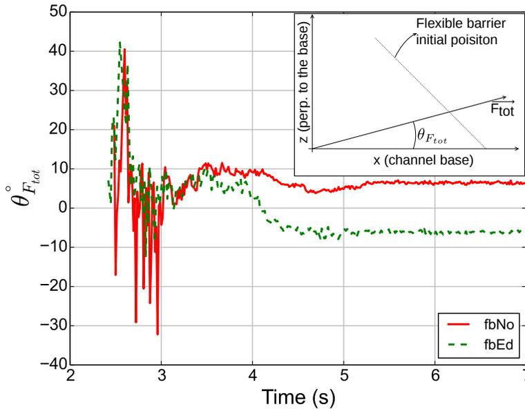
**Figure 4.15:** The evolution with time of the direction of the total force vector with respect to the channel base for two cases: a flexible barrier without energy dissipators (fbNo) and a flexible barrier with energy dissipators (fbEd). Inset: schematic representation of the total force vector direction with respect to the initial position of the barrier and the channel bed
