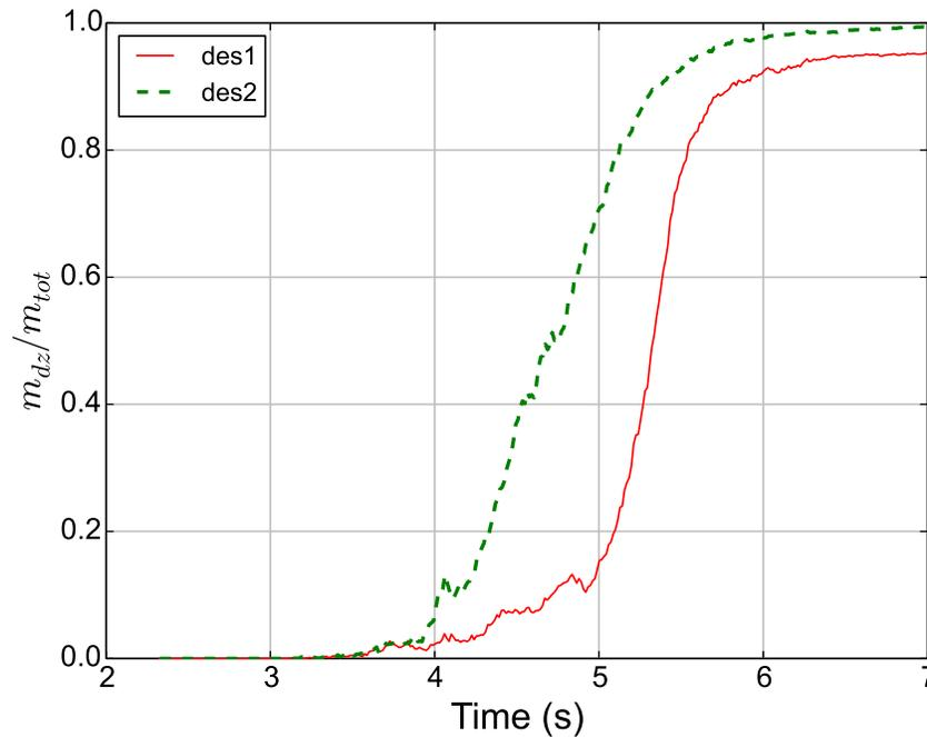
**Figure 5.19:** Evolution of the dead zone mass for two different configurations of the lateral cables: lateral cables connected to energy dissipators ( $des_1$ ) and lateral cables connected directly to the anchors ( $des_2$ )
