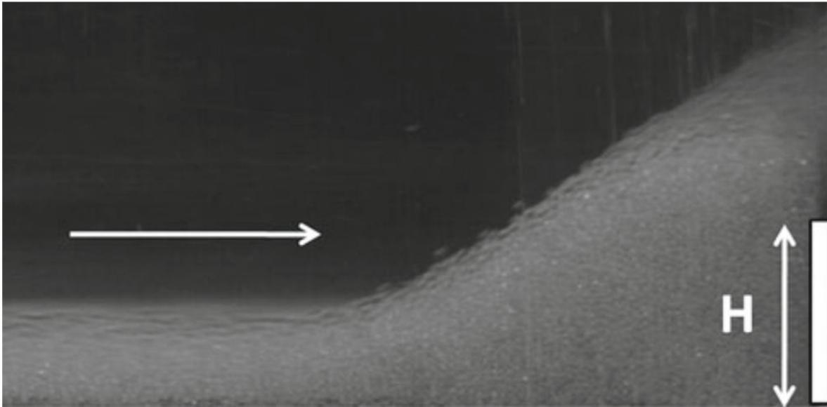
*Figure 2.3: A triangular dead zone is formed upstream of a rigid wall in which moving particles overflow it. The white horizontal arrow indicates the incoming flow direction which is made of glass beads (after [Caccamo et al., 2012](#))*
