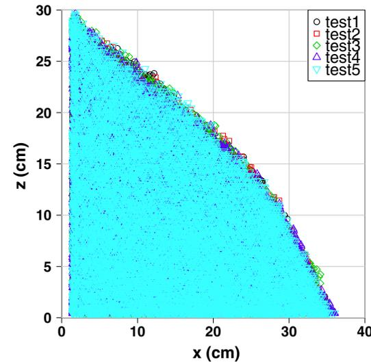
**Fig. 19** The final deposit shape for five tests that have the same initial conditions (test L44-H15- $\alpha 40^\circ$ )
