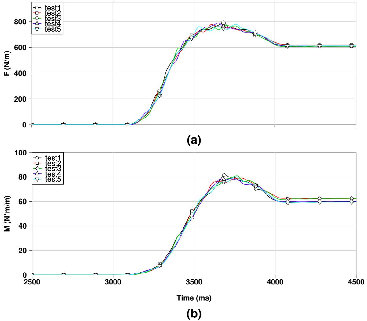
Figure 3.22: Time history of the evolution of total normal force and bending moment (at the toe) for five tests that have the same initial conditions (test L44-H15- $\alpha$ 40°): (a) Total normal force, (b) Total bending moment
