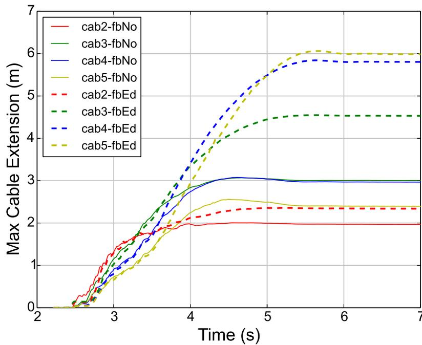
**Figure 4.21:** The evolution with time of the maximum extension of main cables in the direction of the flow for two cases: a flexible barrier without energy dissipators (fbNo) and a flexible barrier with energy dissipators (fbEd)
