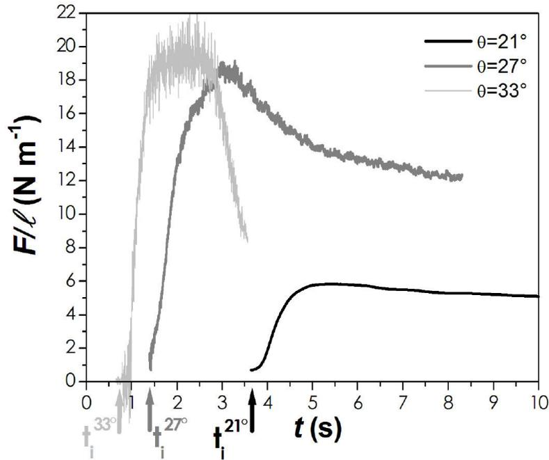
**Figure 4.32:** Force per unit width measured on a wall impacted by a granular flow (made of beads) versus time  $t$  for three slope inclinations:  $\alpha = 21^\circ$ ,  $27^\circ$  and  $33^\circ$  (after [Faug et al., 2011](#))
