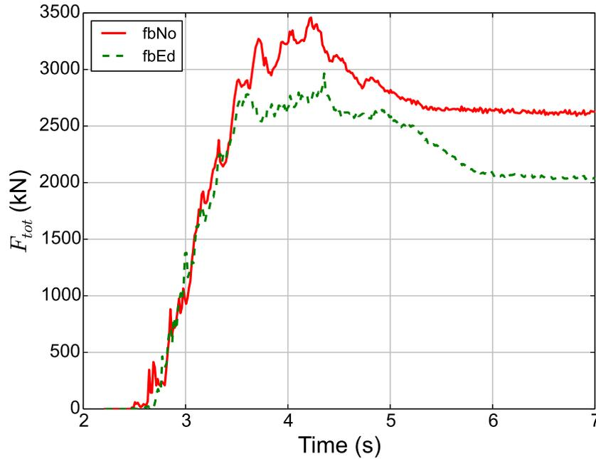
**Figure 4.14:** The evolution with time of the total force applied on the barrier for two cases: a flexible barrier without energy dissipators (fbNo) and a flexible barrier with energy dissipators (fbEd)
