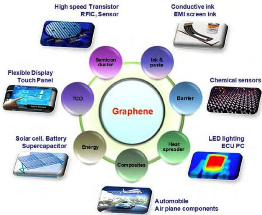
Figure 2.5. Overview of applications of graphene in different sectors ranging from conductive ink to chemical sensors, light emitting devices, composites, energy, touch panels and high frequency electronics. 38
