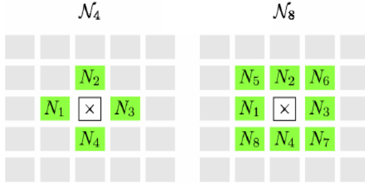
Figure 2.6-Structuring elements in Mathematical morphology
