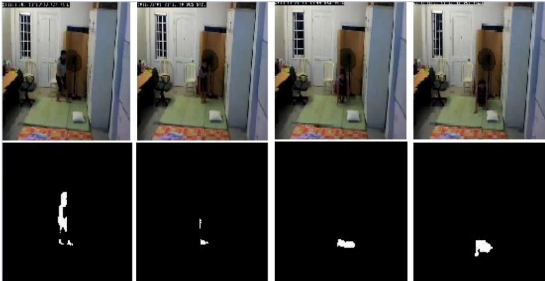
Figure 2.26-Extracted object under not good environment's brightness
