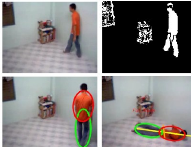
Figure 2.4-Detecting the fall by video analysis
