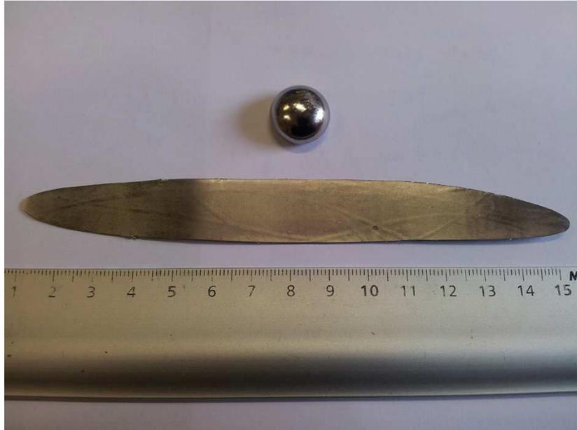
Fig. 3.26  $Ti_{74}Nb_{26}$  as-melted ingot and subjected to 94% reduction ratio of cold rolling.
