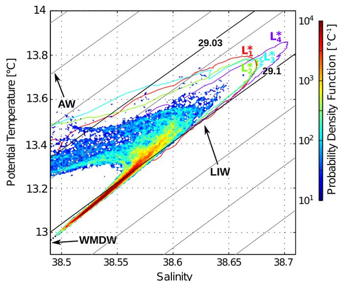
**Figure 4.** Volumetric  $\theta/S$  diagram with the main water masses (AW, LIW, and WMDW) made up by all the profiles (down to 1000 m) collected during the four glider deployments revealing the SCV  $L_i^*$ . The empirical probability density function was normalized such as its integral in the  $\theta/S$  space equals to unity. The colored lines labeled by  $L_i^*$  are associated with the profiles carried out within the core of the four SCVs. Slanted lines represent isopycnals.
