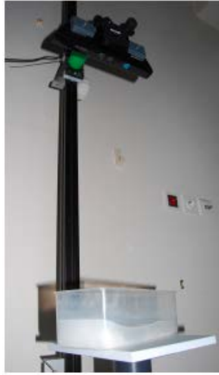
FIGURE 3.9 – Experimental setup with the Kinect depth sensor
