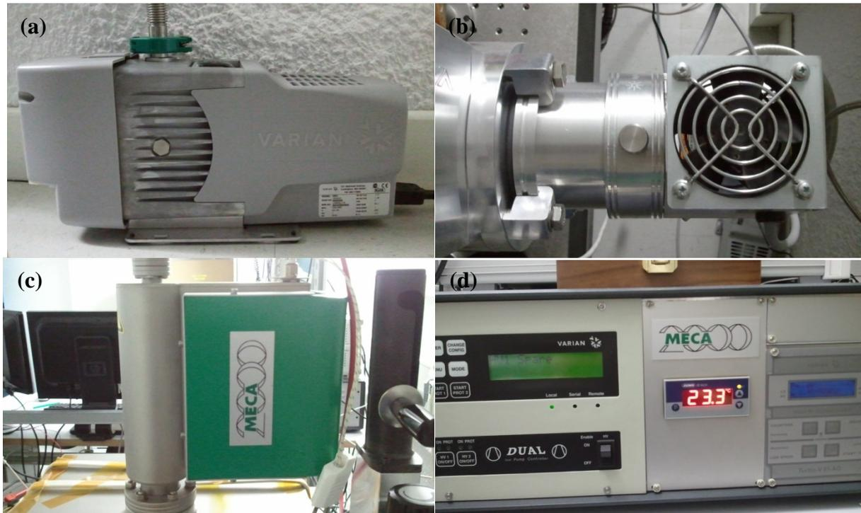
*Figure A.13. Vacuum pumps used to create vacuum in the chamber: (a) The primary pump (IDP-3, Varian), (b) the secondary pump (V 81-M, Agilent Technologies) with the cooling fan and vent valve visible, (c) the ion pump (custom made, MECA 2000). The primary pump is activated by a switch on the pump, while the primary and secondary pumps are operated from (d) the control box, which contains controller for both ion pump (left hand-side) and turbo pump (right hand-side).*
