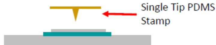
*Figure 4.8. Illustration of a method used to increase the contact quality between the plate and the base. After the micro-masonry process, the plate was pressed along the circumference of the cavity with a single-tip PDMS stamp. It was shown that although this method might reduce plate delamination, it is still dependent on the operator's skill.*
