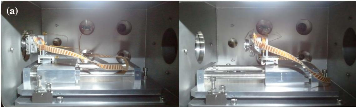
Figure A.10. The sample stage located inside the vacuum chamber. (a) Base pushed completely towards the optical window, ready for optical measurement. (b) Base retracted for sample placement.
