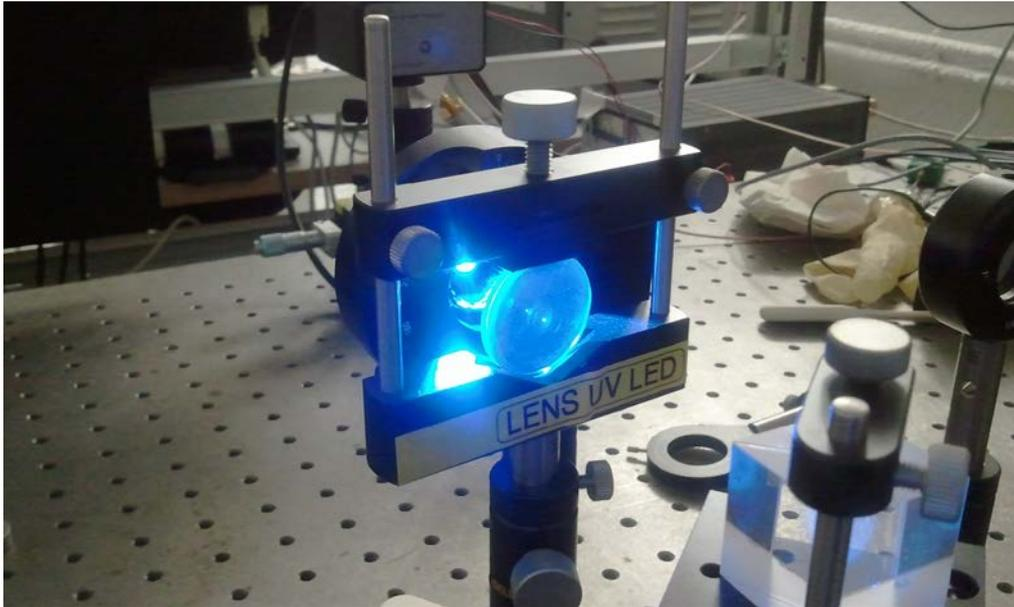
*Figure A.8. The LED used for sample illumination, along with the focusing lens.*
