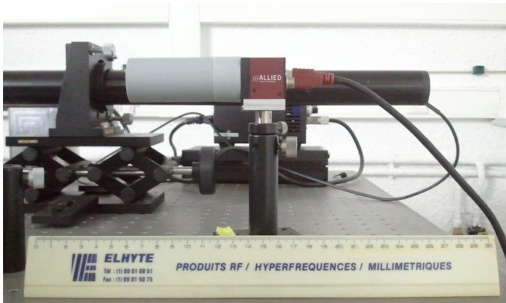
*Figure A.7. The CCD camera used for sample imaging and beam focusing, GUPPY from Allied Vision. The cable is connected directly to the PC using firewire interface, which also acts as the power line. The stand is not fixed to the optical table to accommodate different focus length of magnifying lenses in front of it.*
