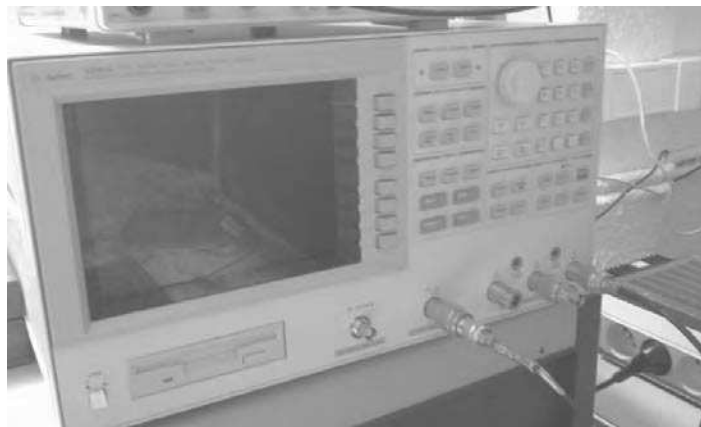
Figure A.4. The spectrum/network analyzer used to process the measurement signal from the photodiode (Agilent 4395A).
