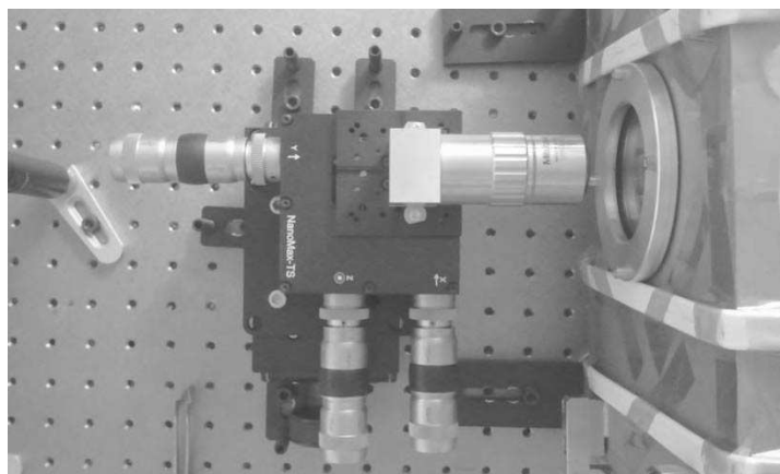
Figure A.6. Microscope lens used to focus the laser beam onto the sample (placed inside the measurement chamber). The lens is mounted on a micrometer holder for fine-tuning. Note the measurement chamber on the right side, with the optical window and kapton tape holding the heating elements used for chamber cleaning.
