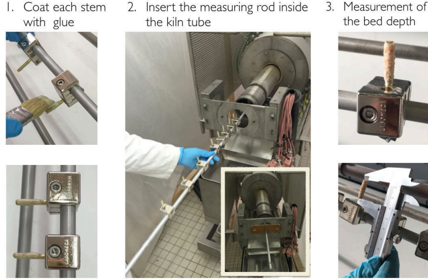
Figure 2.14: Experimental procedure for the bed depth measurement.
