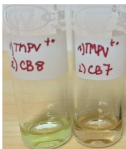
Figure 34. Solutions of \text{TV}^{3(\bullet+)} and \text{CB}[8] (no precipitation, green colour, left) and \text{TV}^{3(\bullet+)} and \text{CB}[7] (precipitation, reddish colour, right).
