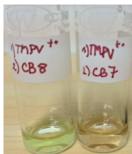
Figure 34. Solutions of \text{TV}^{3(\bullet+)} and CB[8] (no precipitation, green colour, left) and \text{TV}^{3(\bullet+)} and CB[7] (precipitation, reddish colour, right).
