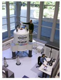
Figure 1.8: NMR spectrometer for the study of the structure of molecules via quantum magnetic effects such as Zeeman energy level splitting.
