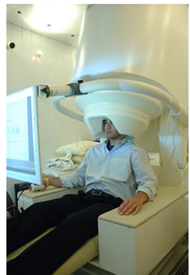
Figure 1.7: MEG machine in a magnetically shielded room (MSR).
