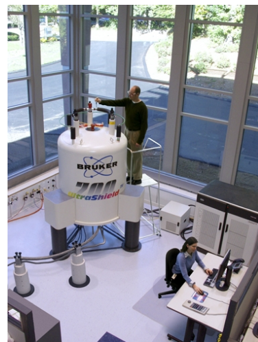
Figure 1.8: NMR spectrometer for the study of the structure of molecules via quantum magnetic effects such as Zeeman energy level splitting.
