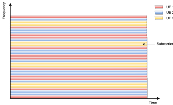
Fig. 2.3 Subcarrier in OFDMA
