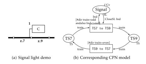
Figure 3.19 – A Petri net representation of signal light
