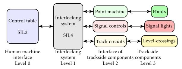
Figure 2.11 – The general architecture of a signal centre
