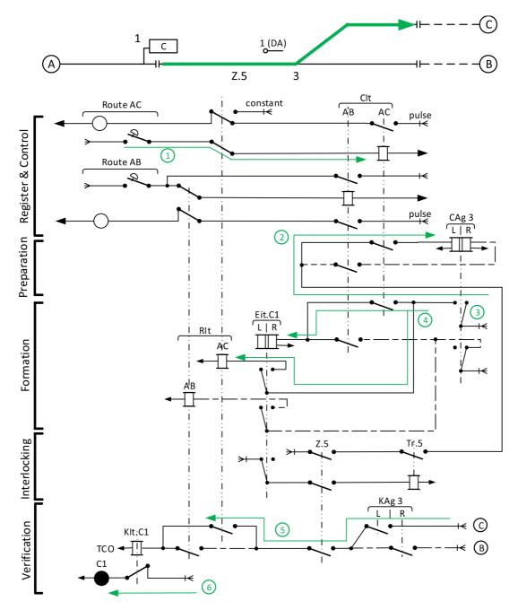
Figure 2.12 – An example of PRS type railway interlocking system
