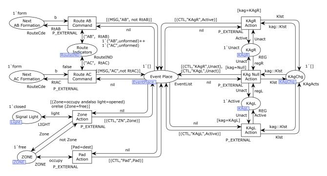
Figure 3.38 – coloured Petri net model of test layer
