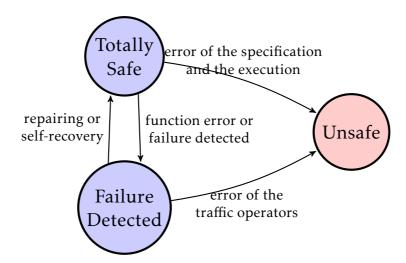
Figure 2.2 – Impact of reliability of the overall safety of a signalling system
