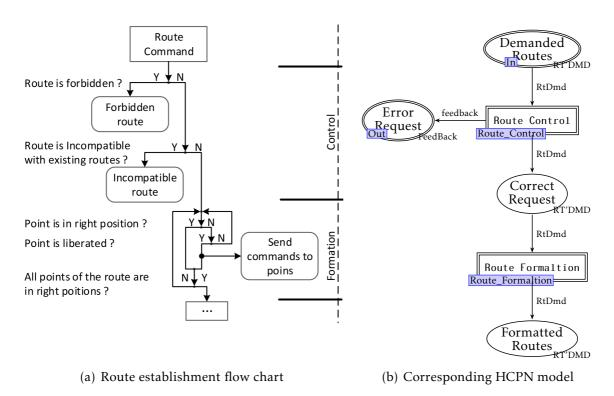
Figure 3.15 – Example of mapping signalling operations (1)
