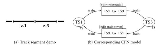
Figure 3.17 – A Petri net representation of track segments
