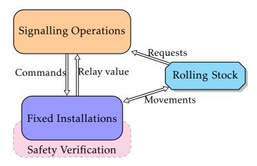
Figure 3.12 – Specification framework of railway interlocking system
