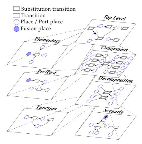
Figure 3.14 – Hierarchical model structure of signalling operation
