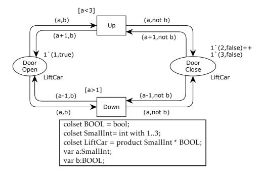
Figure 4.6 – Coloured Petri net of an elevator
