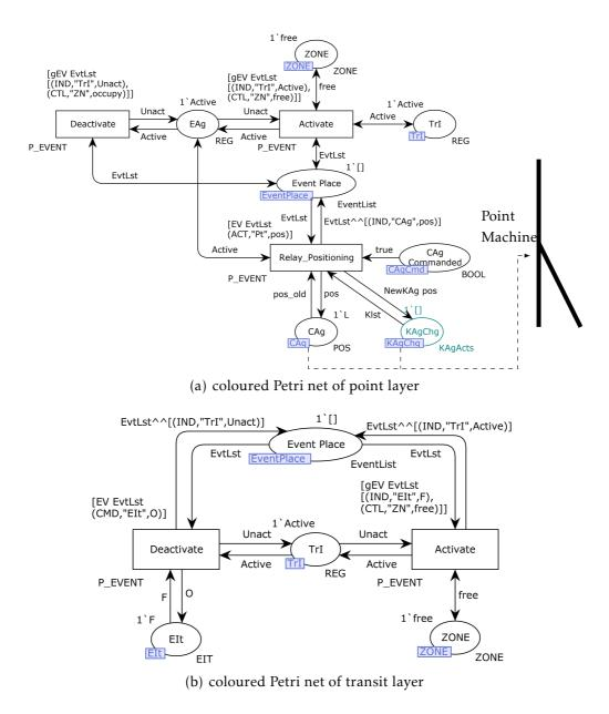
Figure 3.36 – coloured Petri net model of point control
