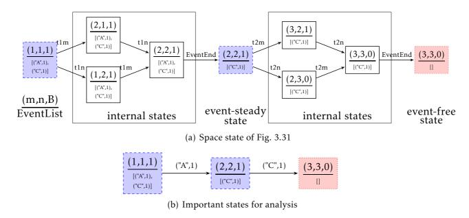
Figure 3.32 – Simplification rules of system space state
