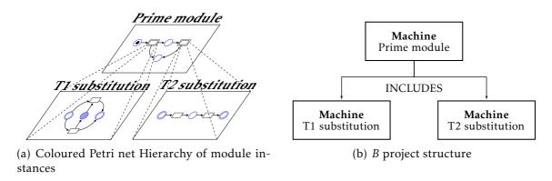
Figure 4.11 – Comparison of hierarchy structure between coloured Petri nets and B machines
