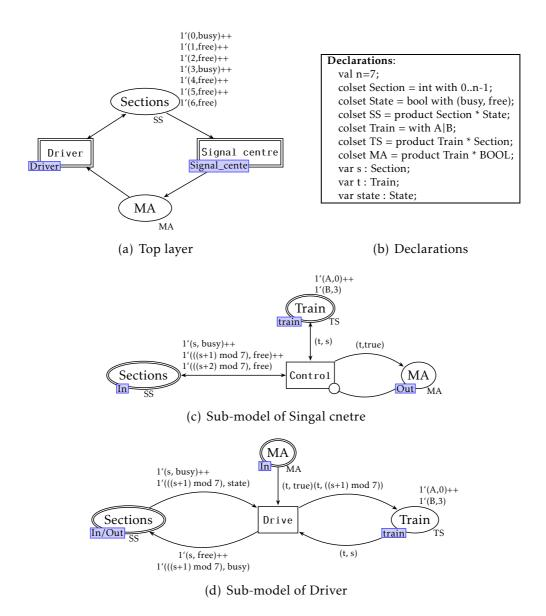
Figure 3.7 – The hierarchical coloured Petri net model of the circular railway with a signal centre
