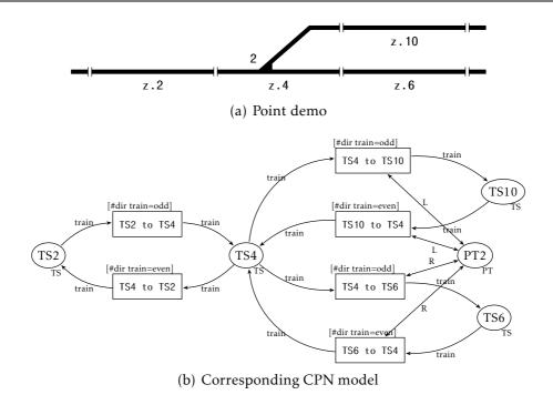
Figure 3.18 – A Petri net representation of point component
