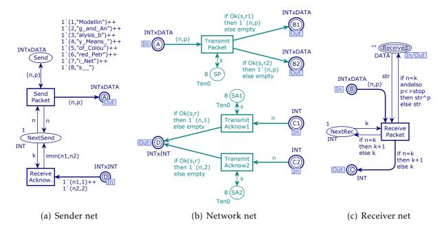
Figure 4.14 – Sub-nets of the hierarchical protocol model
