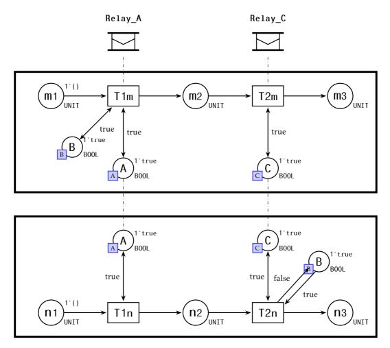
Figure 3.28 – Modelling problem I: synchronous firing
