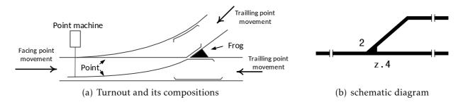
Figure 2.7 – Components of turnout
